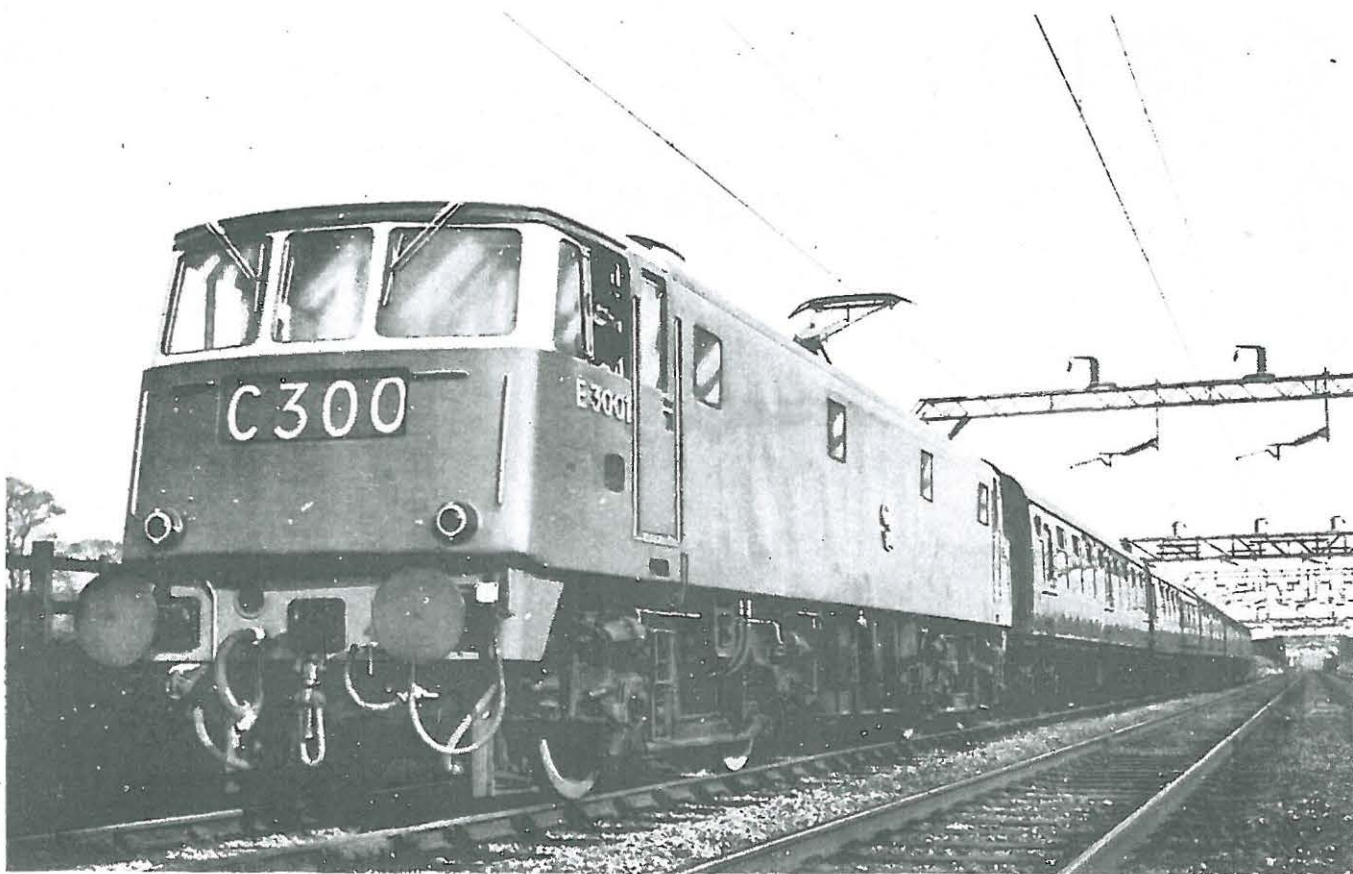
Thirty-five complete 3,300-h.p. 25-kV a.c. locomotives, and forty sets of electrical equipment are being supplied by the AEI Traction Division to British Railways
