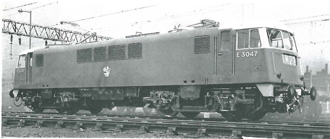
General view of locomotive showing trailing pantograph in operating position
