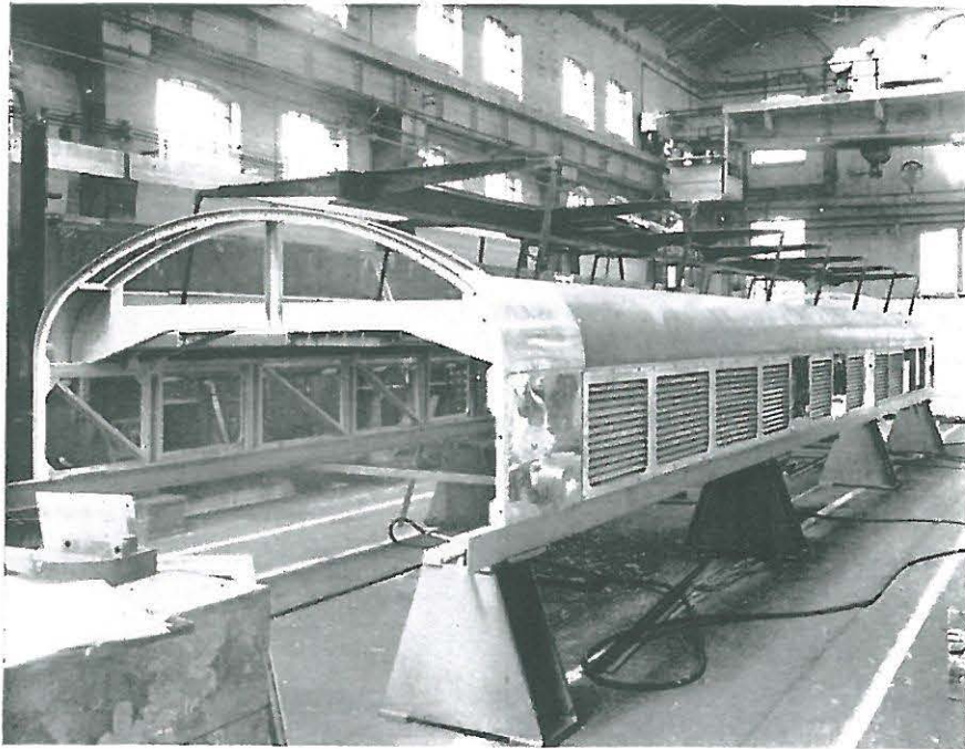
Complete roof and top bodysides made as a light removable unit
