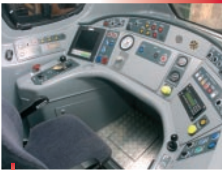
The Pendolino train includes an ergonomic driver cab and easy-to-use driver machine interface for operating the TASS tilt technology
