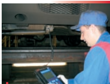
A maintenance technician carries out vibration analysis on the train
