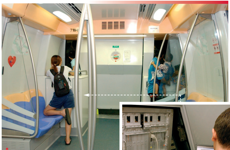
The new, smaller modules of the MASTRIA on-board ATC equipment allow for a train design with more passenger space
