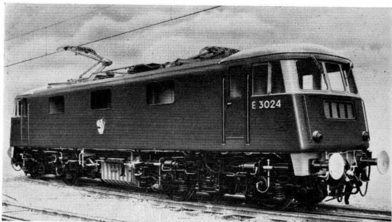
One of fifteen 'ENGLISH ELECTRIC' 3,000 hp 25 kV 50 cycle electric locomotives being supplied to British Railways
