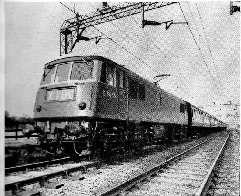
GEC 25 kV 3,300 hp locomotive
