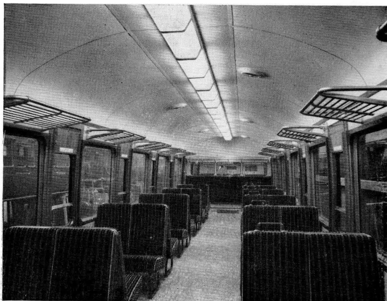
Fluorescent lighting operated by transistor-inverters from 110 V dc supply
