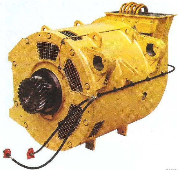
The three-phase-traction-motor of the E 120
