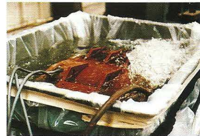
Traction motor (G352BY) undergoing insulation proving tests at 750 V and 3500 rev/min while submerged in a water tank.
