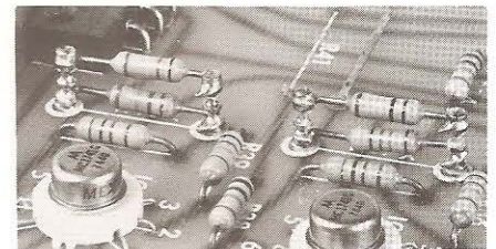
Close up of turret pins on which calibrating resistances are mounted when on test.
