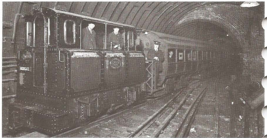
(Above) An early electric locomotive on London's first tube railway. Locomotives similar to this were supplied by GEC in 1890 and continued in service until the 1920s.
